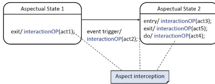
Fig. 3. Extended state-based join point model.
