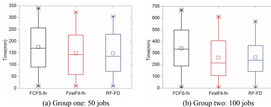
Fig. 5. The boxplot of the two groups. It contains the minimum, maximum, mean and median value of the turnaround time.
