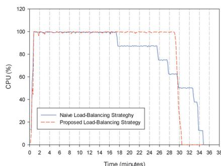
Fig. 3. Comparison of CPU utilization during execution for 8 sub-jobs.
