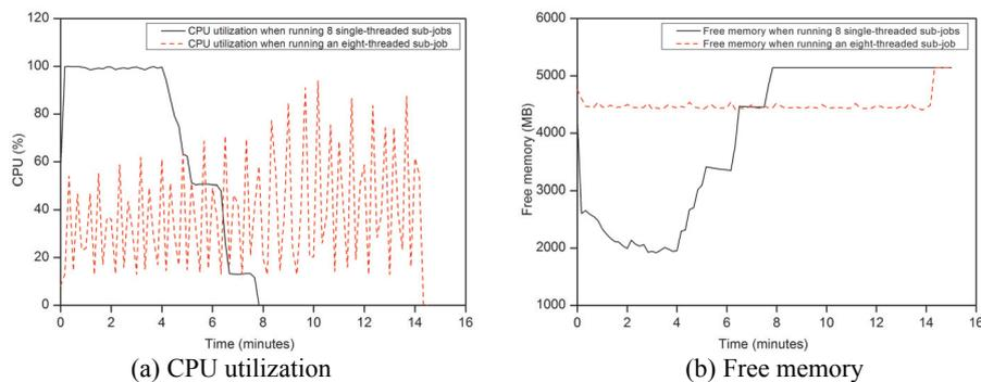
Fig. 1. CPU utilization and free memory during the execution of 8 single-threaded sub-jobs and an eight-threaded sub-job.
