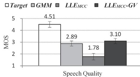
**Fig. 5.** Subjective test results of the speech converted by  $GMM$ ,  $LLE_{MCC}$  and  $LLE_{MCC-GV}$ . Error bars indicate 95% confidence intervals. “*Target*” denotes the analysis-synthesized target speech.
