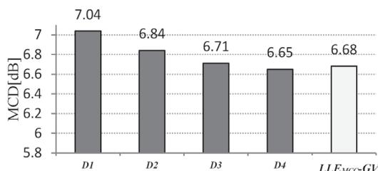
Fig. 6. The average MCD values of *MTO-LLE* with different sizes of dictionaries (*D1*~*D4*) and *LLE<sub>MCC</sub>-GV*. The MCD value before conversion is 9.45dB.
