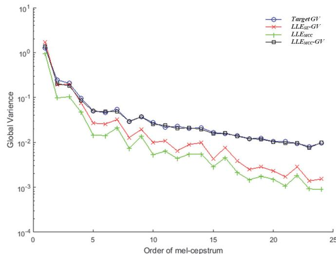
Fig. 4. The average GV measurements of the converted MCCs given by the three proposed SC systems (i.e.,  $LLE_{MCC-GV}$ ,  $LLE_{SE-GV}$ , and  $LLE_{MCC}$ ) and the natural MCCs of the target speech (i.e., *Target GV*).
