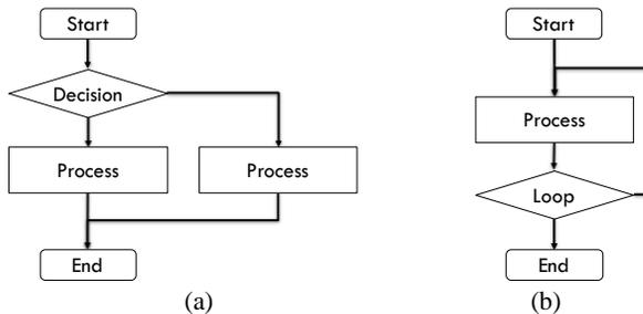
Fig. 3. Using Decision (a) and Loop (b).
