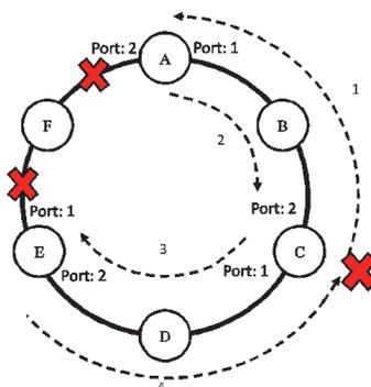
Fig. 3. Loop avoidance in LPFR when double link failure occurs.
