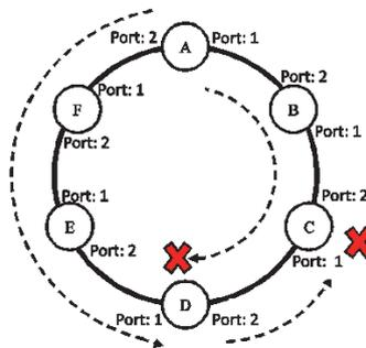
Fig. 2. Operation of LPFR under multi/broadcast traffic type.
