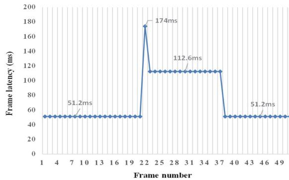
Fig. 8. Frame latency under different cases for the first simulation’s scenario.
