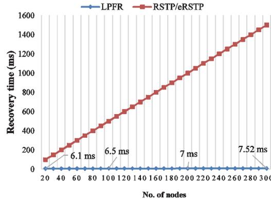
Fig. 7. Recovery time of LPFR compared to the RSTP/eRSTP.
