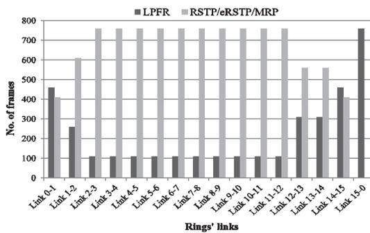
Fig. 9. Frame distribution among the network links of Fig. 4 during the second simulation’s scenario.
