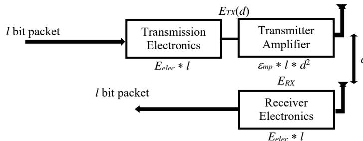
Fig. 1. Block diagram of first order energy model.
