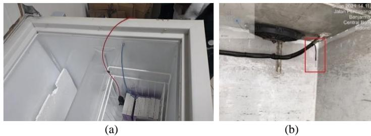
Fig. 3. Temperature probe installation in (a) chillers and (b) trucks.
