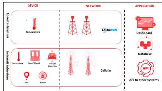
Fig. 2. Device-network-application system architecture.
