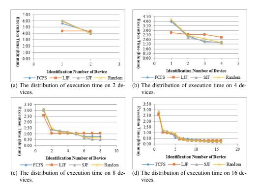
Fig. 10. The distributions of test execution time on different number of devices.
