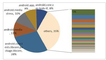
Fig. 5. The percentage of text execution for CTS test package.
