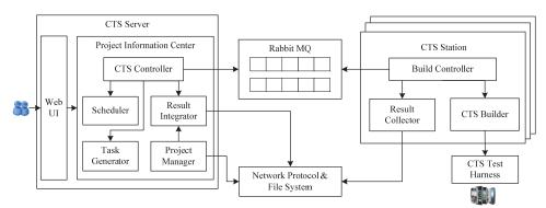
Fig. 6. The system architecture of the AndroidCTS.
