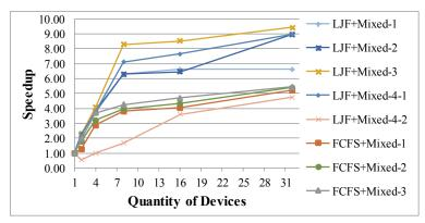
Fig. 12. The speedup of mixed partitioning methods with FCFS and LJF.
