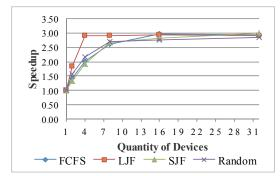
Fig. 9. The speedup for package partition under different scheduling.
