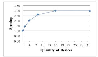
Fig. 8. The speedup for package partition under FCFS scheduling.
