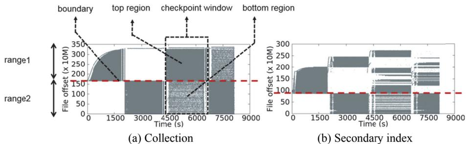
Fig. 3. Write patterns of various file types in WiredTiger with Linkbench benchmark.
