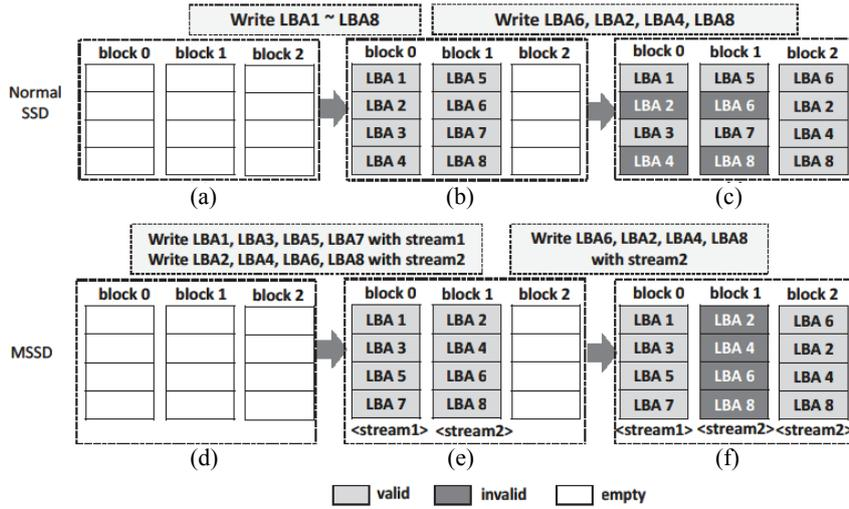
Fig. 1. Comparison between normal SSD and multi-streamed SSD.
