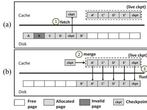
Fig. 2. Reusing data at checkpoint time in WiredTiger.
