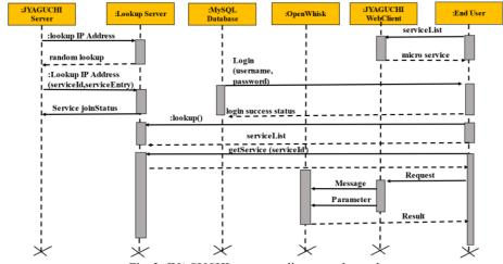
Fig. 3. JYAGUCHI sequence diagram enhanced.
