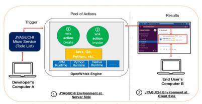
Fig. 7. Integration of serverless architecture in JYAGUCHI.
