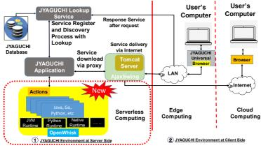
Fig. 2. JYAGUCHI ClouEdge (Cloud-Edge) and serverless environment.
