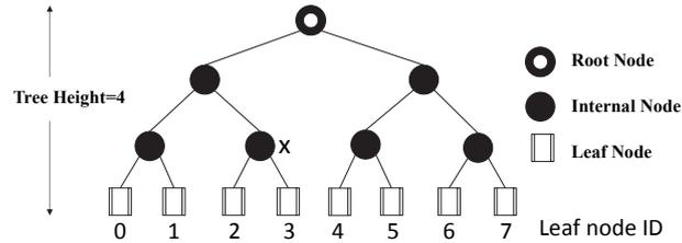
Fig. 5. An FBHTree that is four nodes high.
