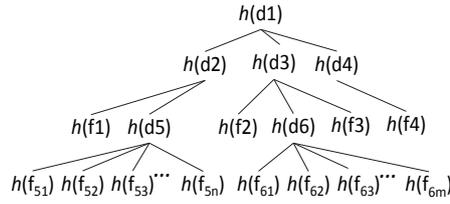
Fig. 3. The hash tree corresponding to the file directory in Fig. 2.
