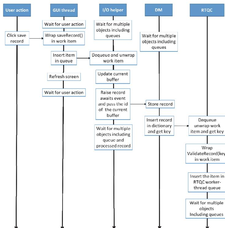
Fig. 8. The process of record transmission.
