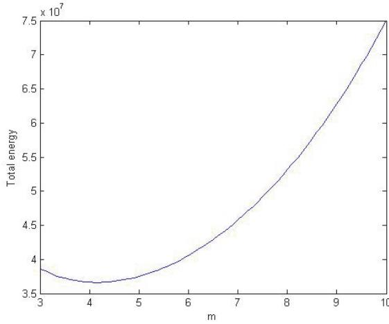
Fig. 2. The relationship between  $m$  (representing the CPU frequency) and the total energy consumption.
