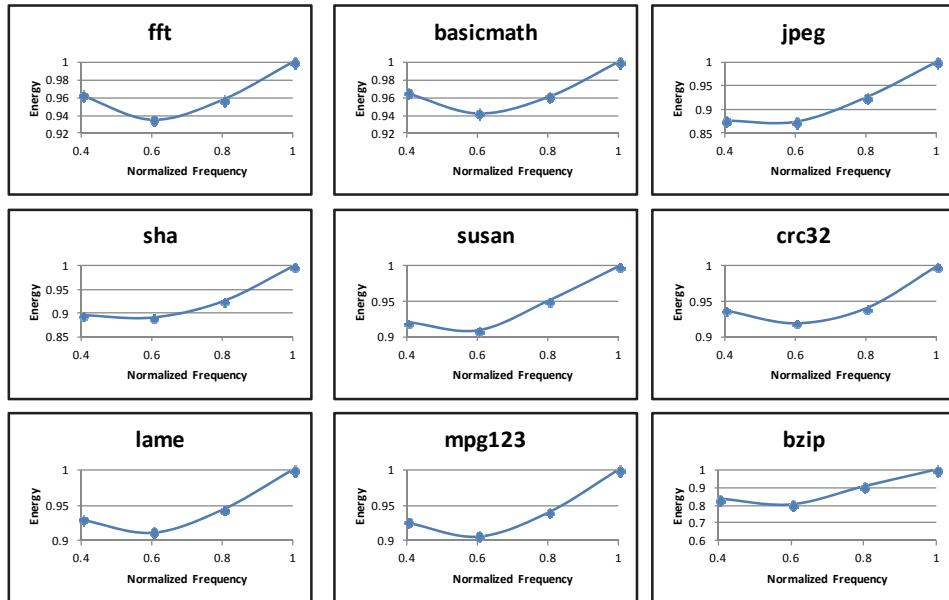
Fig. 1. Energy consumption for different frequencies. The CPU speed and the energy are normalized with respect to that of the highest frequency supported by the processor.
