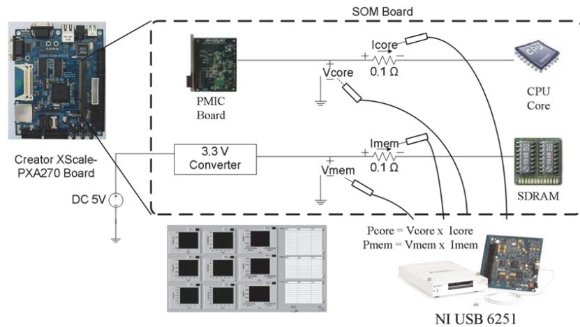
Fig. 7. Measurements of the Creator PXA270 components.
