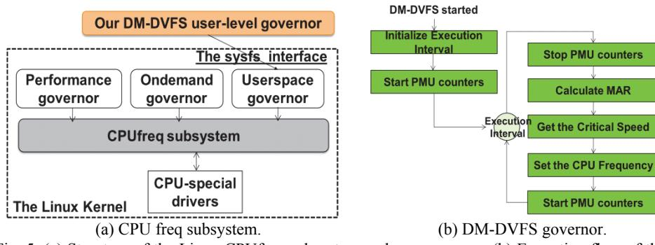
Fig. 5. (a) Structure of the Linux CPUfreq subsystem and our governor; (b) Execution flow of the DM-DVFS.
