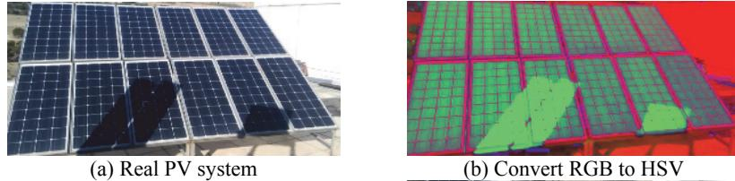
Fig. 19. The outputs obtained by image processing at time  $t+1$  for TCT type.
