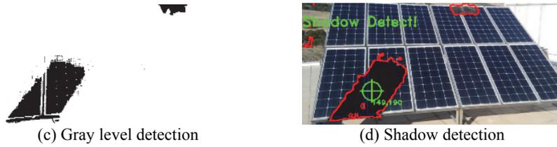
Fig. 18. (Cont'd) The outputs obtained by image processing at time  $t$  for TCT type.
