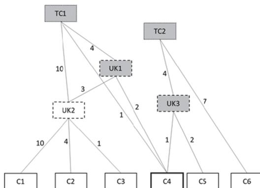
Fig. 8. A coupling diagram with how many times a module has been used.
