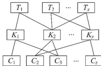
Fig. 2. A general call graph of test cases, keywords, and components. A vertex  $T_i$  denotes a test case, a vertex  $K_j$  denotes a keyword, and a vertex  $C_i$  denotes a component on which an action is performed.
