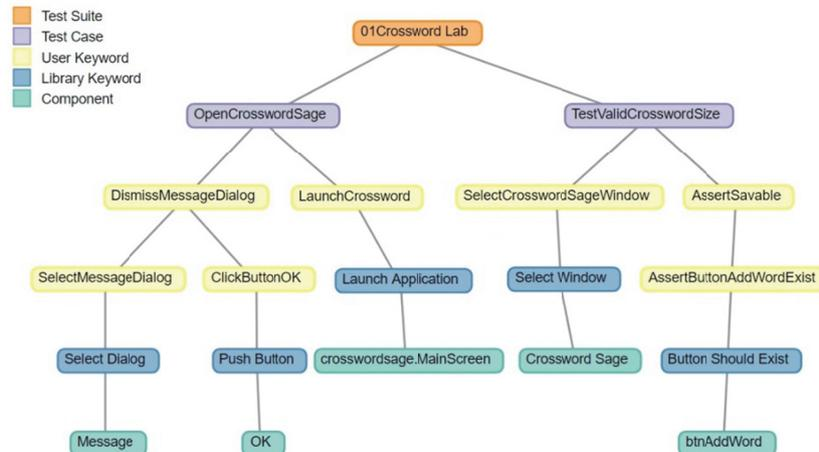
Fig. 7. An example of the TS-TC-K-C diagram.
