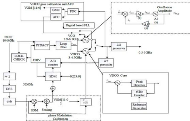
Fig. 2. Detailed block diagram of the hybrid PLL.
