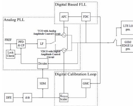
Fig. 1. Multi-standard frequency synthesizer based on the proposed hybrid PLL.
