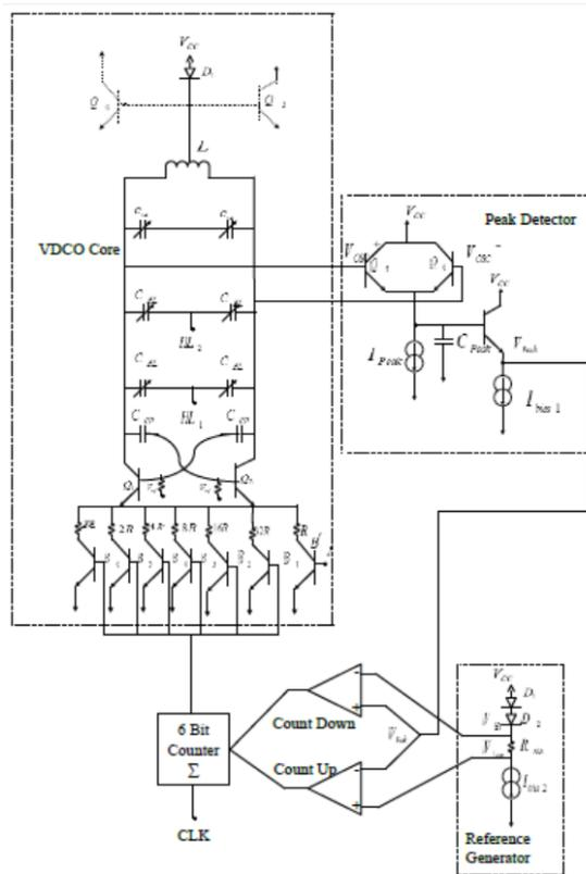
Fig. 4. VDCO topology with adjustable degeneration resistors placed in a digital automatic-amplitude control loop.
