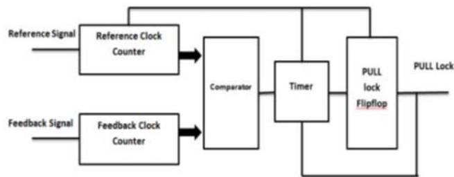
Fig. 3. Block diagram of the lock check.
