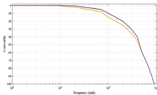
Fig. 7. AC response of the fourth-order loop filter.
