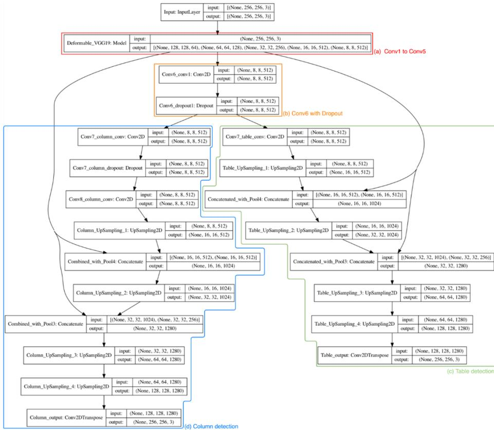
Fig. 2. Detail stages of TD-DCNN.
