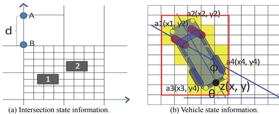
Fig. 3. Meshing at the intersection.
