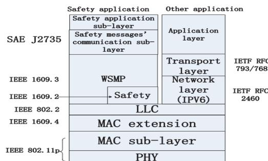
Fig. 2. The DSRC communication protocol stack.
