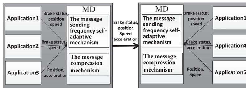
Fig. 1. The structure of optimal designed communication sub-layer.
