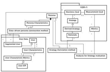
Fig. 3. UML class diagram-based relations of attributes in ID3P.
