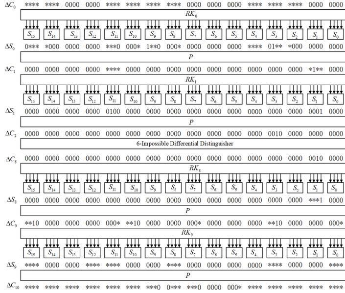
Fig. 4. Impossible difference attack of BORON.
