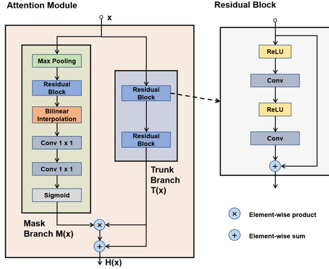
Fig. 1. The structure of the attention module.
