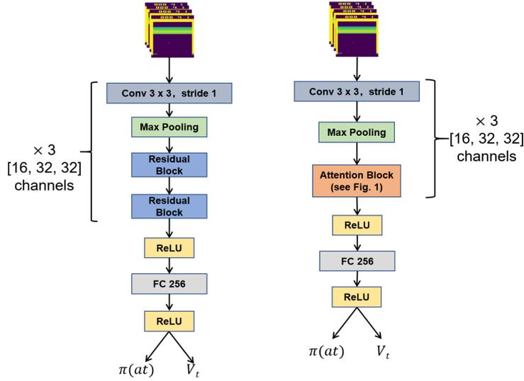
Fig. 2. Model architecture; (Left) IMPALA, which is same to the network structure proposed in study [2]; (Right) DRARL, using one attention block (explained in Section 3.1) instead of two residual blocks.
