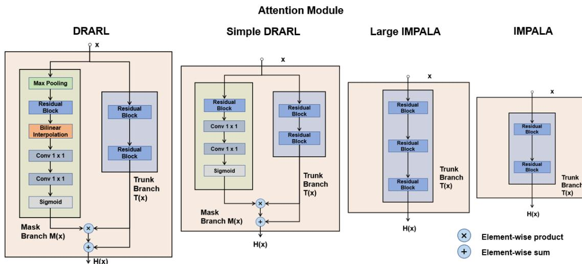
Fig. 5. The structure of a single network module (instead of each attention module in Fig 1) of DRARL, IMPALA and two new alternatives.
