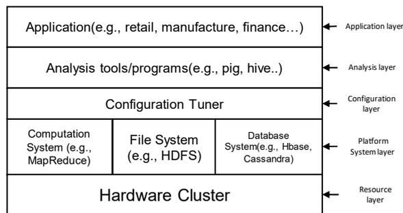
Fig. 2. The overview of a big data platform with configuration layer.
