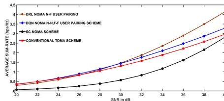
Fig. 6. Convergence variation during the training process. Fig. 7. Average Sum rate versus SNR in dB for various user pairing schemes.
