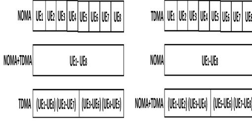
Fig. 3. Schematic representation of the N-F pairing scheme.
