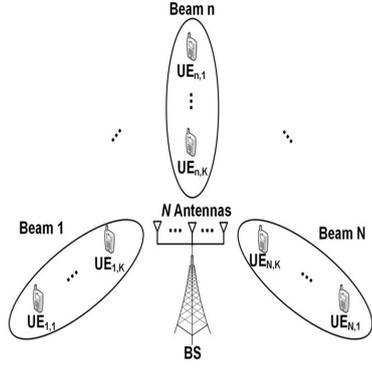
Fig. 1. Schematic representation of the D/L NOMA with multiple antennas.
