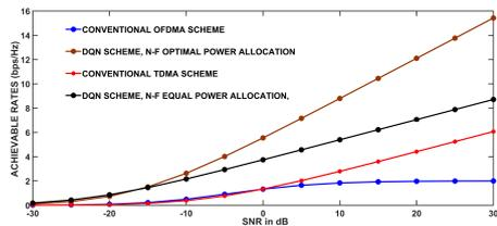
Fig. 10. Performance comparison between the equal and optimal power allocation factors.
