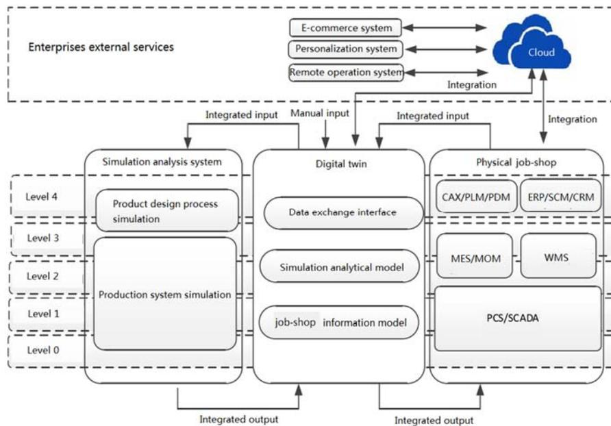
Note: SCADA: Supervisory control and data acquisition; WMS: Warehouse management system; CAX: Computer-aided X; MOM: Material on machine; PCS: Process control system
