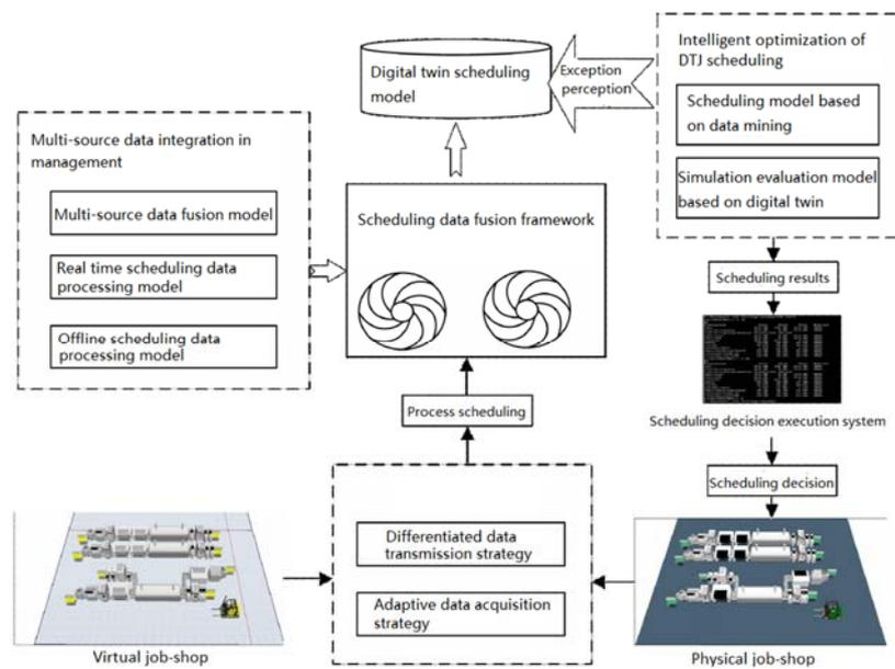
Fig. 1. The architecture of the DTJ.
