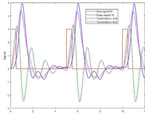
Fig. 4. Input, output and TSs in the communication system of Ex. 1 for a pulse train.
