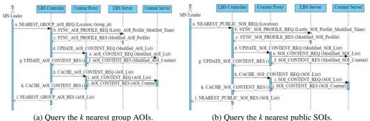
(a) Query the k hearest group AOIS. (b) Query the k hearest public SOIS. Fig. 6. The message flow diagrams for the control schemes of different querying functions in the narrator mode, part B.
