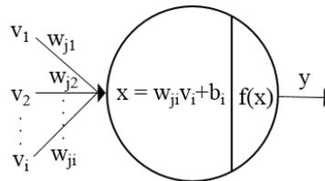
Fig. 2. Basic operation in a perceptron.
