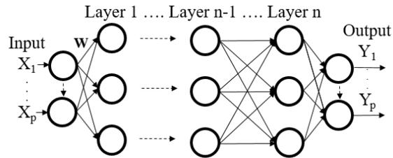
Fig. 6. Sequentially adding hidden layers to the deep feedforward neural network is set up to evaluate the optimizers performance for vanishing gradient analysis.
