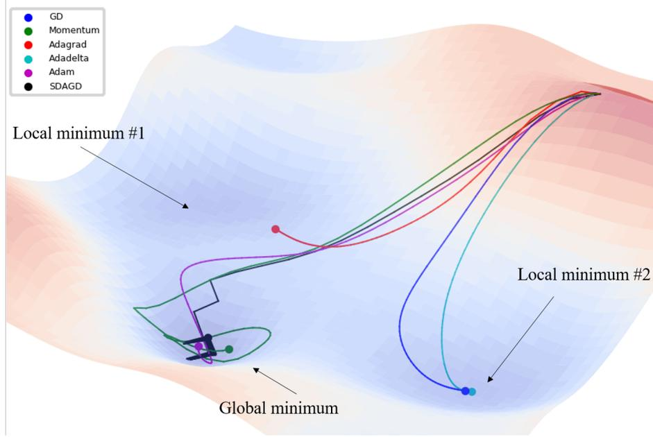
Fig. 3. A hilly error surface with two local minimums and one global minimum.
