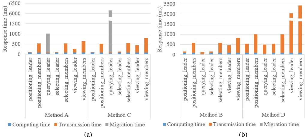
Fig. 14. (a) The response time using method A and method C ( $n = 2$ ); (b) The response time using method A and method D ( $n = 2$ ).
