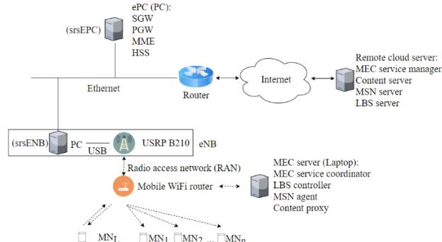
Fig. 12. The networking configuration of the experiment.
