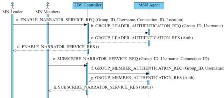
Fig. 2. The message flow diagram of the control scheme for the enabling service function and the subscribing service function.
