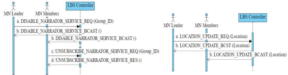
Fig. 3. The message flow diagram of the control scheme for the disabling service function and the unsubscribing service function.
