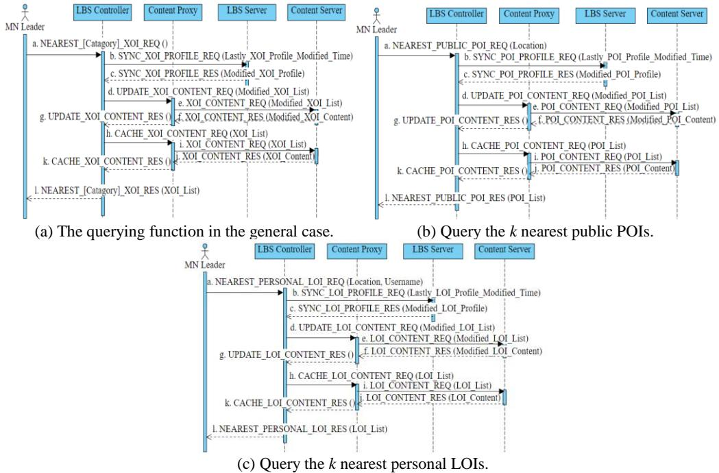
Fig. 5. The message flow diagrams for the control schemes of different querying functions in the narrator mode, part A.
