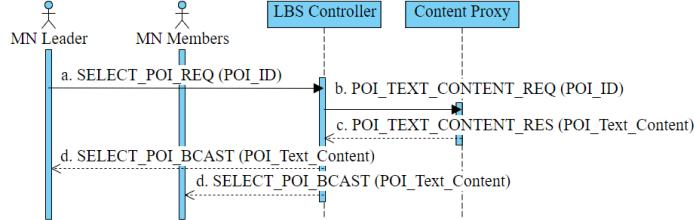
Fig. 7. The message flow diagram of the control scheme for the selecting POI function in the narrator mode.
