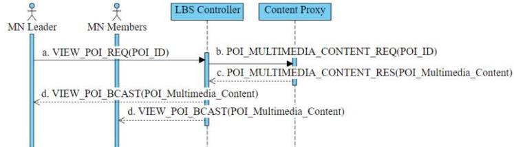
Fig. 8. The message flow diagram of the control scheme for the viewing function in the narrator mode.
