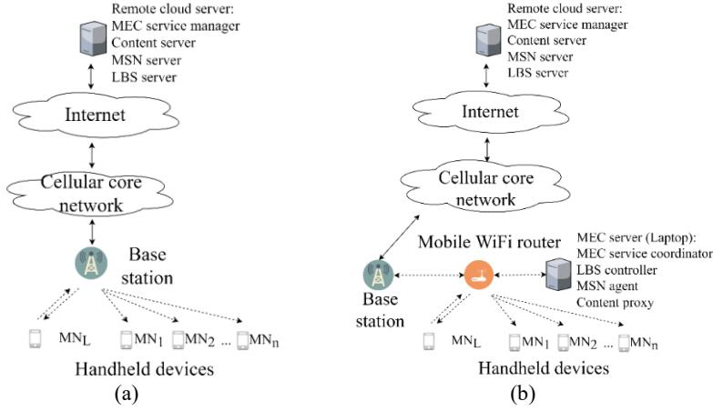
Fig. 1. The networking configuration of downloading text and multimedia contents of POIs from (a) the remote cloud server; and (b) the MEC server.
