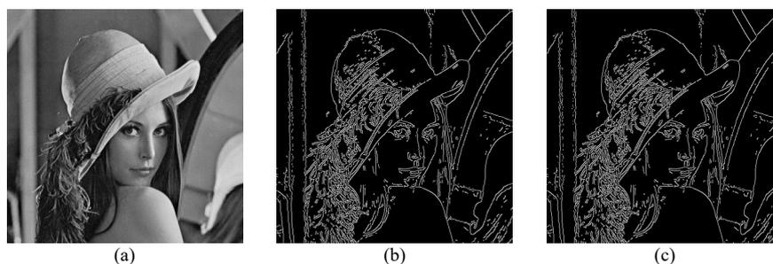
Fig. 9. Proposed Canny results with software programme and VLSI circuit; (a) Original “image01”; (b) “image01” by software; and (c) “image01” by circuit.
