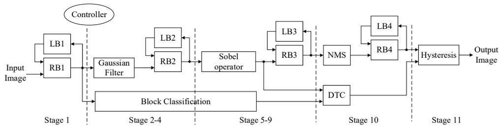
Fig. 2. Block diagram of hardware architecture for our Canny mechanism.
