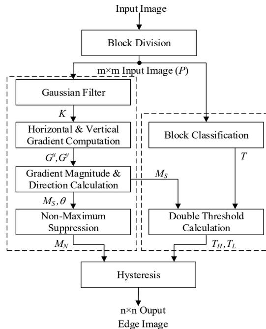
Fig. 1. Flow diagram of the Canny mechanism.
