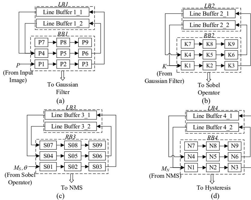
Fig. 6. Architecture of line buffers and the register banks: (a) for Gaussian filter; (b) for Sobel operator; (c) for NMS; and (d) for Hysteresis.
