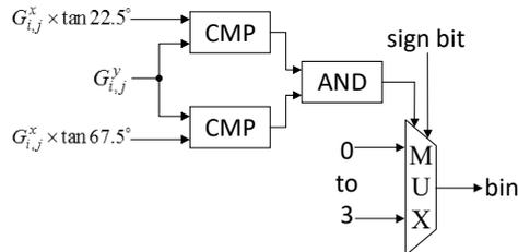
Fig. 5. Architecture of  $G_{i,j}^x \times \tan 22.5^\circ \leq G_{i,j}^y < G_{i,j}^x \times \tan 67.5^\circ$ .
