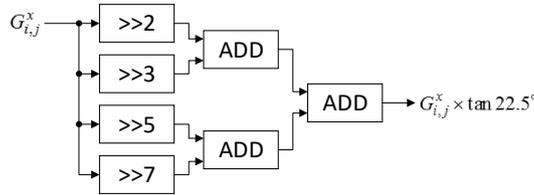
Fig. 4. Architecture of  $G_{i,j}^x \times \tan 22.5^\circ$ .
