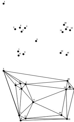
Fig. 1. Delaunay triangulation of 15 points [30].
