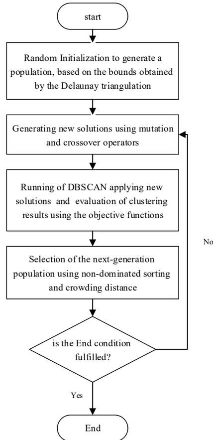
Fig. 2. The flowchart of MOGA-DBSCAN.
