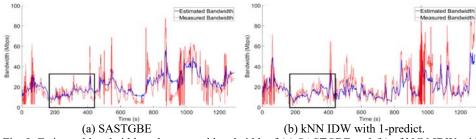
Fig. 9. Estimated bandwidth and measured bandwidth of (a) SASTGBE and (b) of kNN IDW with 1-predict.
