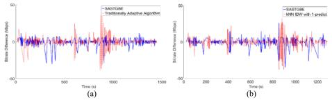
Fig. 11. Presentation bitrate difference considering playback suspending; (a) SASTGBE vs. the traditional method; (b) SASTGBE vs. the kNN IDW with 1-predict method.
