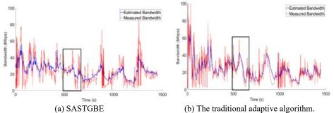
Fig. 7. Estimated bandwidth and measured bandwidth of (a) SASTGBE and (b) the traditional adaptive algorithm.
