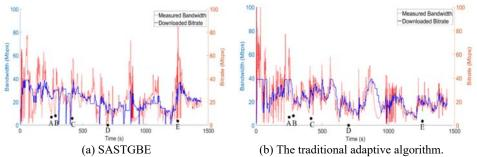
Fig. 8. Measured bandwidth and downloaded bitrate of (a) SASTGBE and (b) of the traditional adaptive algorithm.
