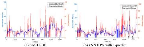
Fig. 10. Measured bandwidth and downloaded bitrate of (a) SASTGBE and (b) of kNN IDW with 1-predict.
