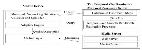
Fig. 1. System components of the proposed streaming architecture.
