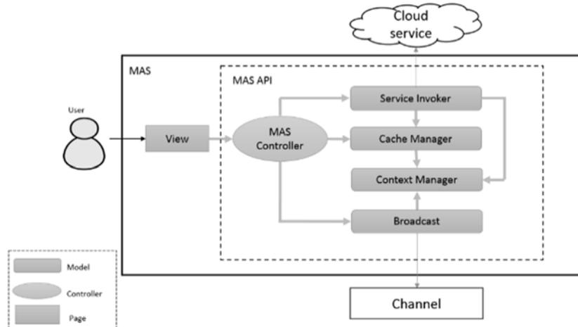
Fig. 2. MASA system architecture.
