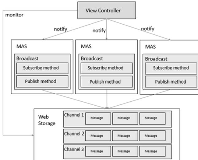
Fig. 4. Architecture for the broadcast mechanism.
