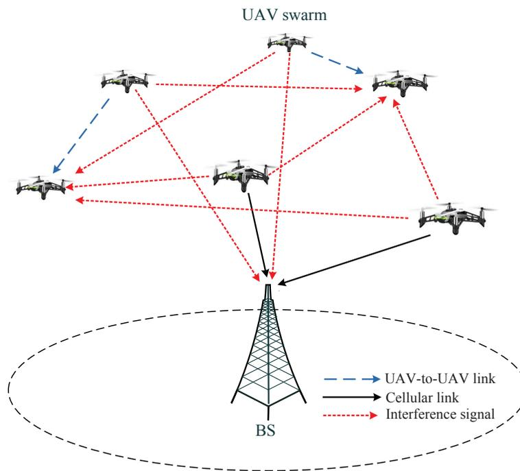
Fig. 1. Network model consisting of a BS and a UAV swarm.
