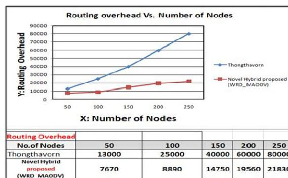
Fig. 7. WRD\_MAODV Routing Overhead (Number of nodes).
