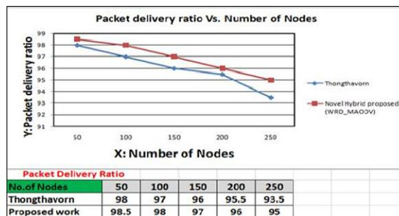
Fig. 6. Packet delivery ratio of WRD\_MAODV (Number of nodes).
