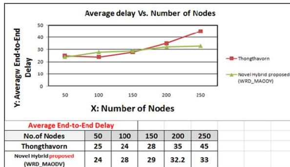
Fig. 5. Average end-to-end delay of WRD\_MAODV (Number of nodes).
