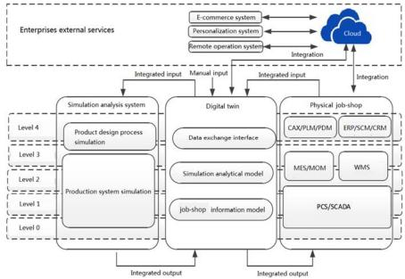
Note: SCADA: Supervisory control and data acquisition; WMS: Warehouse management system; CAX: Computer-aided X; MOM: Material on machine; PCS: Process control system Fig. 3. Information integration architecture.
