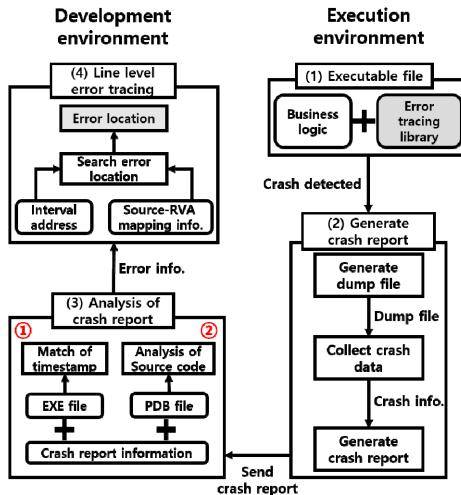
Fig. 4. Overview of crash report generation, analysis, and error tracing methods.
