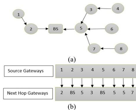
Fig. 2. (a) A sub-graph of WSN; (b) Chromosome representation; Circle Gateway, square base station, arrow direction of flow of data.
