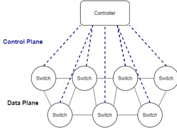
Fig. 1. Software-defined networking (SDN).
