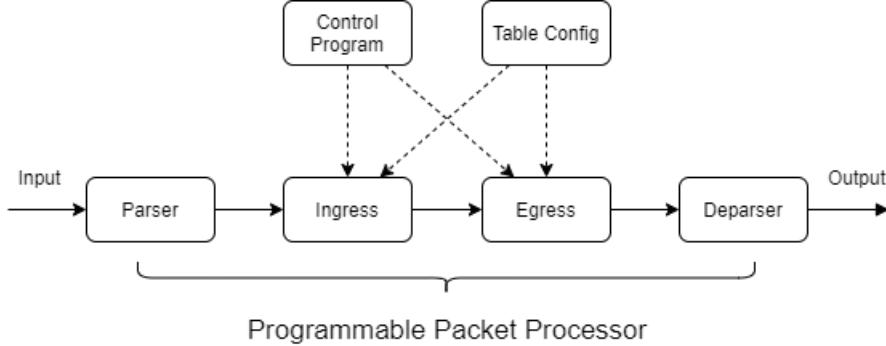
Fig. 2. Protocol-independent packet processor (P4).
