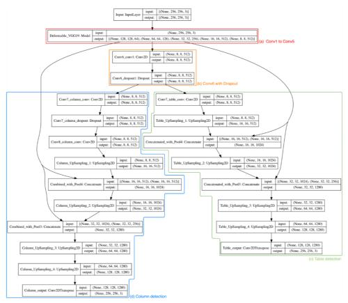
Fig. 2. Detail stages of TD-DCNN.
