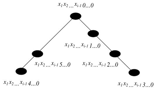
Fig. 5. The transmission pattern used by node  $x_1 x_2 \cdots x_{i-1} 0 \cdots 0$  in step  $i$  of the one-port broadcasting algorithm.
