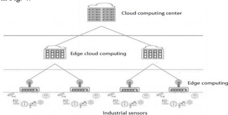
Fig. 4. The structure of edge computing in the physical job-shop.
