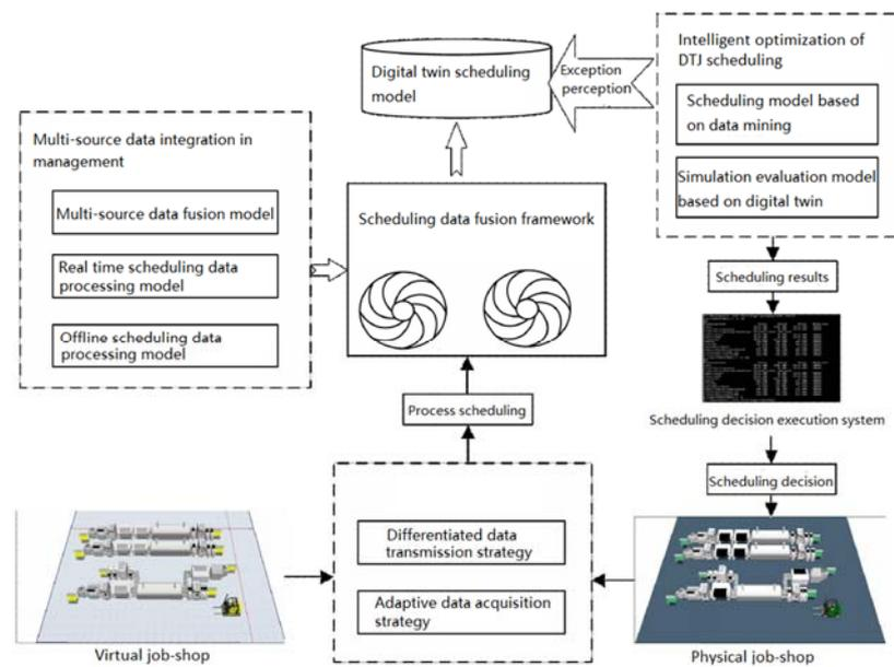
Fig. 1. The architecture of the DTJ.
