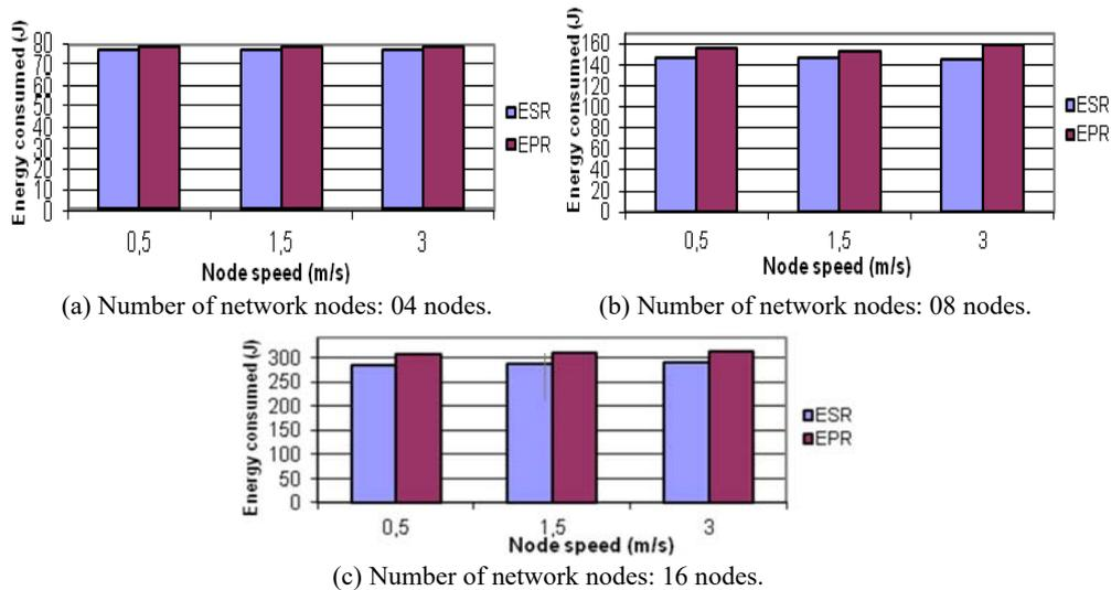
Fig. 5. Energy consumed versus node speed.
