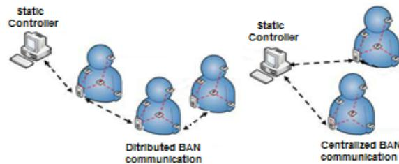
Fig. 2. Centralized and distributed BAN communications.
