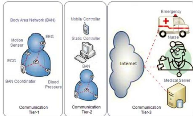
Fig. 1. BAN communication architecture.
