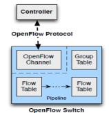
Fig. 1. The OpenFlow Switch architecture.
