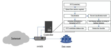
Fig. 2. Our SDN intrusion detection architecture.
