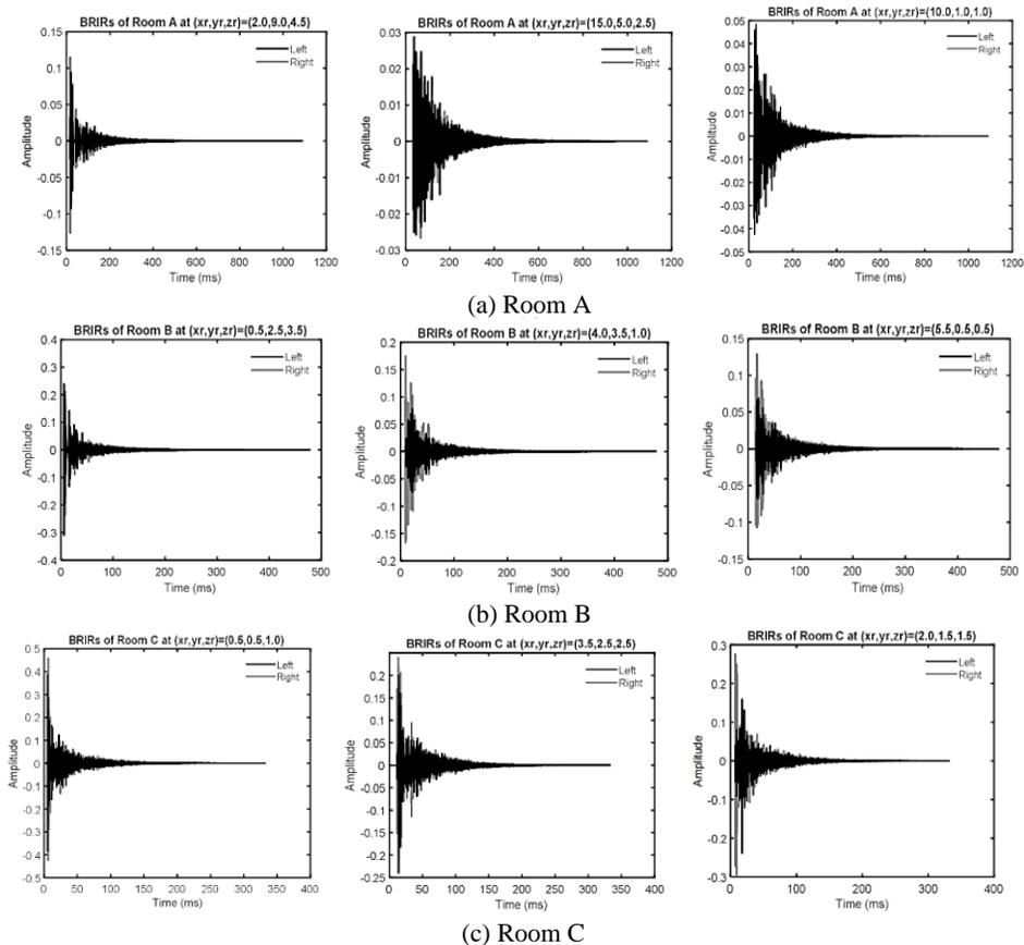
Fig. 5. BRIRs results of the receiver at the three different locations.
