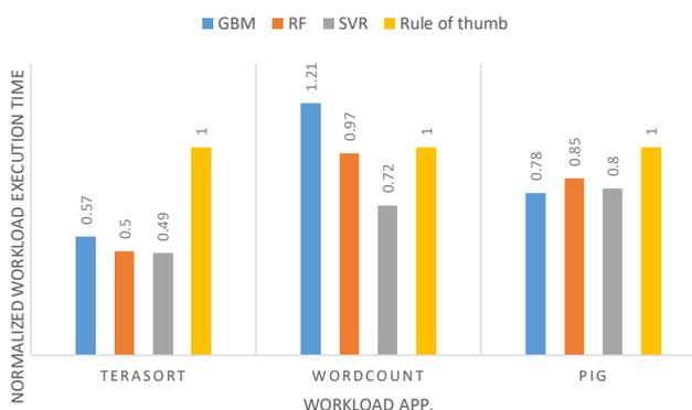
Fig. 11. Normalized workload execution times of different models and workloads.
