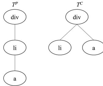
Fig. 7. Soft template error matching when different tree structures generate the same tag sequences.
