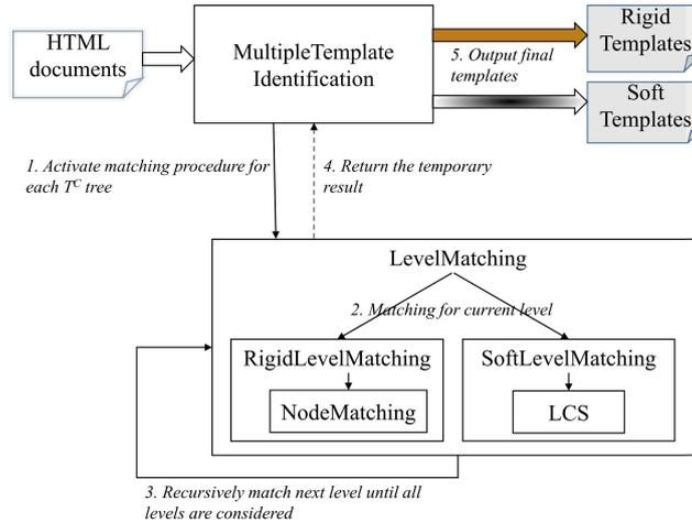
Fig. 4. The workflow of web template identification.
