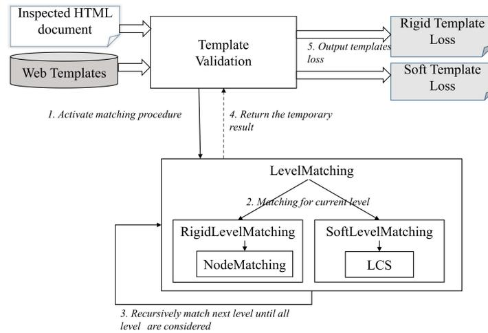
Fig. 9. The workflow of Web template validation.
