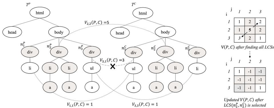
Fig. 8. Soft template wrong order matching: after  $n_2^P$  and  $n_2^C$  were matched, matching between  $n_3^P$  and  $n_1^C$  lead to wrong order matching.
