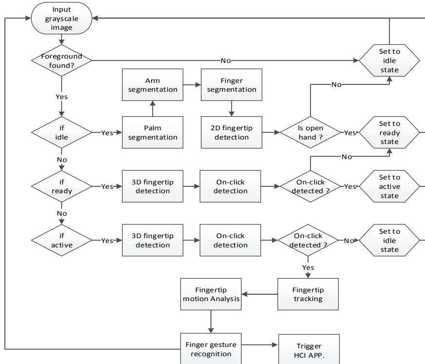
Fig. 2. The overview of system flowchart.
