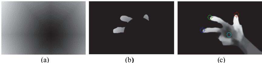
Fig. 6. (a) The  $\mathbf{P}^{DT}$  distance map; (b) The  $\mathbf{P}_{finger}^{DT}$  distance map; (c) The fingertips and the palm center.
