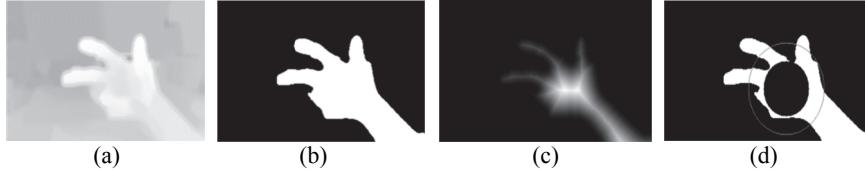
Fig. 5. (a) The input depth image; (b) The binary image  $\mathbf{P}$ ; (c) The distance map  $\mathbf{P}^{DT}$ ; (d) The radius of central circle is  $DT_{max}$ , the radius of larger circle is  $1.5DT_{max}$ .
