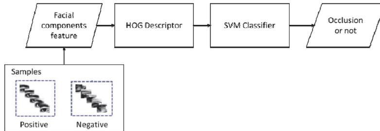
Fig. 7. The occlusion classification procedures of the facial feature.
