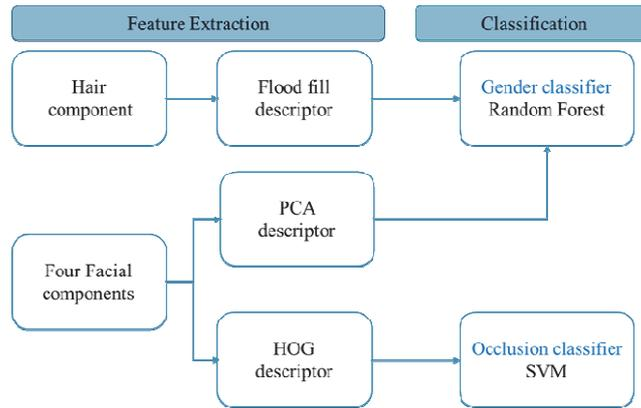
Fig. 5. The relationship between the different feature extractors and classifiers.
