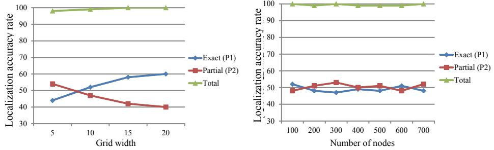
Fig. 6. Localization accuracy of non-grid nodes versus grid width and node density.
