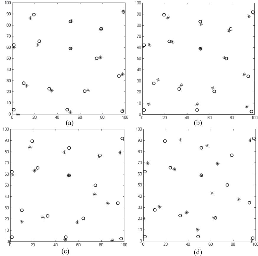
Fig. 5. The established grid coordinate system with  $M = 15$ . The small circles ("o") denote the real coordinates of the nodes and the stars ("\*") represent the calculated grid coordinates after coordinate transformation; (a)  $\psi = 1.7804$ ,  $w = 5$ ; (b)  $\psi = 4.0752$ ,  $w = 10$ ; (c)  $\psi = 4.8085$ ,  $w = 15$ ; (d)  $\psi = 8.4885$ ,  $w = 20$ .
