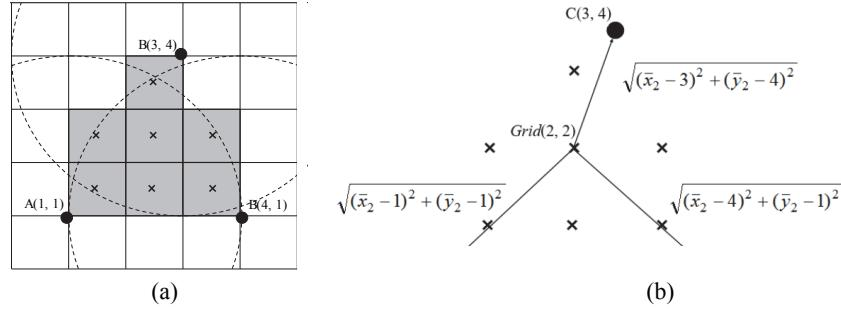
Fig. 3. An illustration of positioning non-grid nodes; (a) The intersection set of grid cells; (b) The distances between grid  $Grid(2, 2)$  and grid nodes  $\{A, B, C\}$ .
