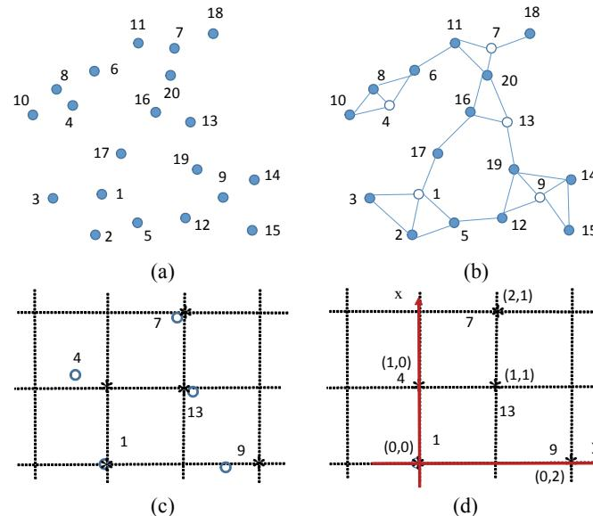
Fig. 1. Grid coordinate system establishment. The small circles ("o") denote the real coordinates of the nodes and the stars ("\*") represent the calculated grid coordinates after coordinate transformation; (a) Distribution of nodes; (b) The constructed graph  $G(V, E)$  and the set of grid nodes for establishing the grid coordinate system; (c) The local grid coordinate system; (d) The transformed grid coordinate system.
