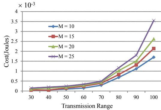
Fig. 7. Energy cost versus transmission range.
